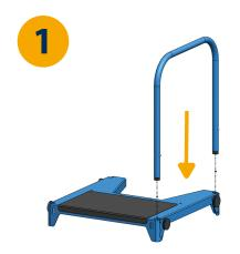
Loosen the 4 knobs on the step stool. Slide one handle into the platform with the button pins facing outward.
