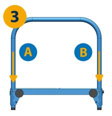
Press in the other button pin and work side to side (A-B) to slide the handle down evenly.
