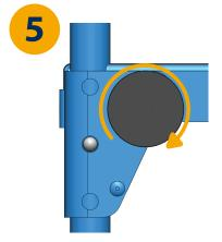
Once at the desired height, tighten the knobs firmly. \* (Clockwise)
