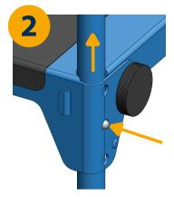
Press button pins in and pull the handle out of the platform. Work side to side incrementally as described step 3 of the assembly instructions to pull the handle out evenly.
