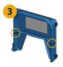
Store handles below the platform. Pull outward on the rubber straps (circled) and wrap them around the handles. Hooks are provided to attach the straps.
