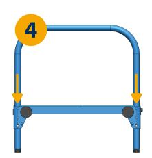
Continue to work side to side until the desired height setting is reached. Ensure the button pins have clicked into place.
